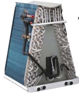
Models with TXV pre-installed in factory are also available Thermostatic Expansion Valve (TXV) simplifies field installation and precisely controls refrigerant flow for efficient cooling.
